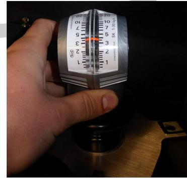
All readings need to be the same. If your throttles are out of balance, you should adjust the throttles with the higher readings. Adjustment can be made via the small bleed screws on
